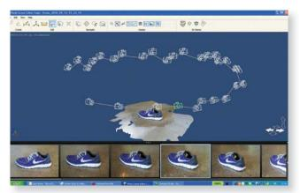
Constructing a 3D scene using 2D photos of an object taken from various angles.
